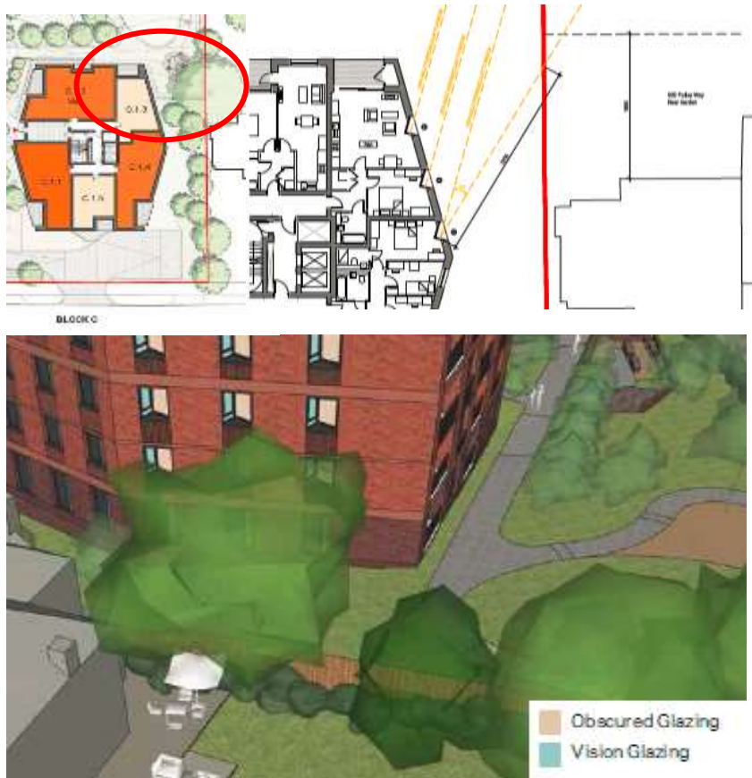
Image 18 – Site Layout planning detailing Block C and 920 Purley Way (top left), close up of inset windows (top right) and CGI visualisation of this approach (bottom)
